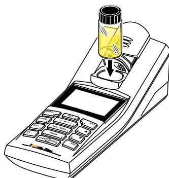
**Inserting a 16 mm cell**
