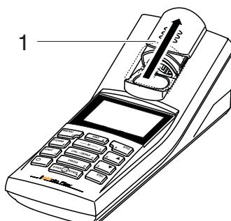
**Inserting a 28 mm cell**
